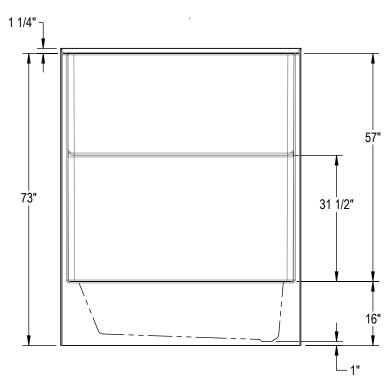
All dimensions are approximate. Structure measurments must be verified against the unit to ensure proper fit.
