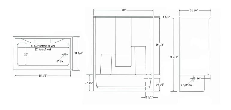
$\textbf{FEATURES} \ \, \text{Dimensional Tolerance} \, \pm \, \textbf{\%}". \, \text{Dimensions needed for site preparation should be measured from the unit. American Bath Group assumes no responsibility for preparatory work.}$
