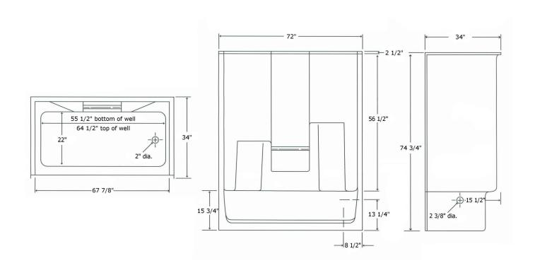
FEATURES Dimensional Tolerance ± %". Dimensions needed for site preparation should be measured from the unit. American Bath Group assumes no responsibility for preparatory work.
