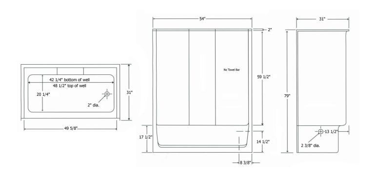
FEATURES Dimensional Tolerance ± %". Dimensions needed for site preparation should be measured from the unit. American Bath Group assumes no responsibility for preparatory work.
