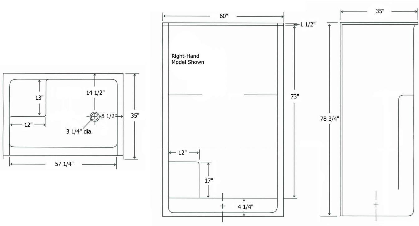
**FEATURES** Dimensional Tolerance ± 3/16". Dimensions needed for site preparation should be measured from the unit. American Bath Group assumes no responsibility for preparatory work.
