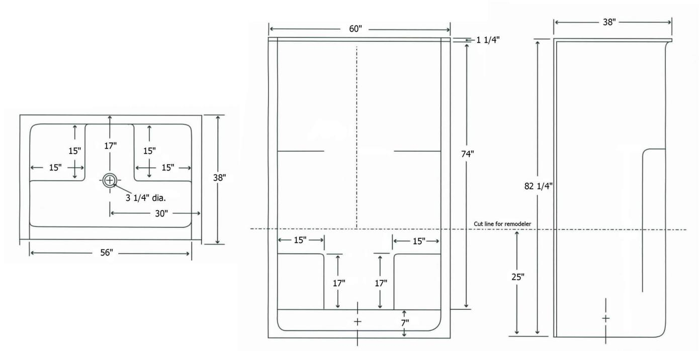
**FEATURES** Dimensional Tolerance  $\pm \frac{3}{16}$ ". Dimensions needed for site preparation should be measured from the unit. American Bath Group assumes no responsibility for preparatory work.
