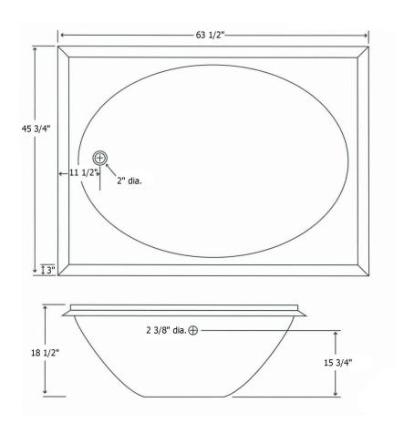
FEATURES Dimensional Tolerance ± %". Dimensions needed for site preparation should be measured from the unit. American Bath Group assumes no responsibility for preparatory work.
