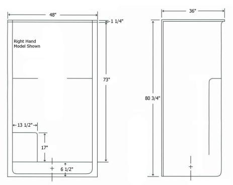
FEATURES Dimensional Tolerance ± %". Dimensions needed for site preparation should be measured from the unit. American Bath Group assumes no responsibility for preparatory work.
