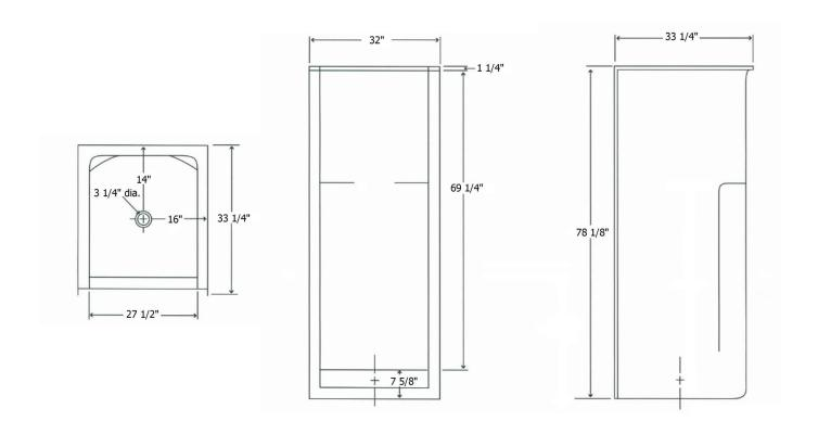
FEATURES Dimensional Tolerance ± %". Dimensions needed for site preparation should be measured from the unit. American Bath Group assumes no responsibility for preparatory work.
